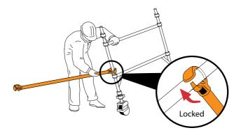
Position the ladder frame as shown and fit the other end of the horizontal brace on to the vertical (just above the bottom rung). Fit a second horizontal brace between the bottom rungs on the other side of the frames to square the tower.
