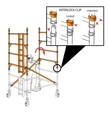
Fit a temporary deck on the lowest rungs. Fit a trapdoor deck on the 4th rung (2.0m) with the trapdoor next to the ladder. Ensure the trapdoor is positioned with the hinges towards the outside of the tower as shown. Climb the ladder and, from the protected trapdoor position, fit guardrails on the 5th and 6th rungs (in that order) on both sides of the platform.
