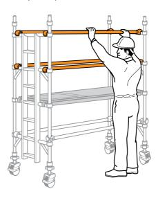
Fit two diagonal braces in opposing directions between the 1st and 3rd rungs. Ensure that the frames are vertical and level by checking with a spirit level and setting the adjustable legs as necessary. Fit stabilisers (see notes on **page 30**). Fit the next pair of end frames and check the frame interlock clips are engaged.
