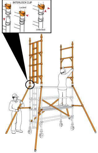
Fit two pairs of diagonal braces in opposing directions between the 3rd and 5th rungs and the 5th and 7th rungs.
