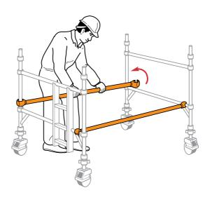
Fit two additional end frames, ensuring the frame interlock clips are engaged. Fit two diagonal braces (blue) in opposing directions, between the 1st and the 3rd rungs. Ensure the frames are vertical and level by checking with a spirit level and setting the adjustable legs as required.
