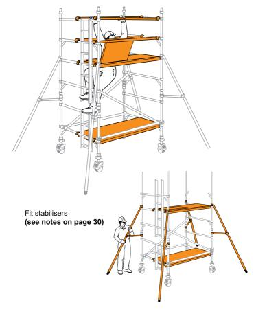
6 Fit the next pair of diagonal braces in opposing directions between the 3rd and 5th rungs. Add two additional end frames.
